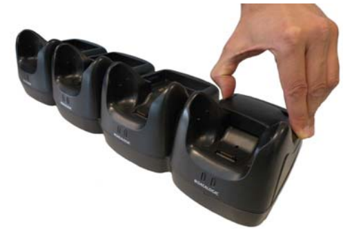
Figure 5 - Spare Battery Removal
