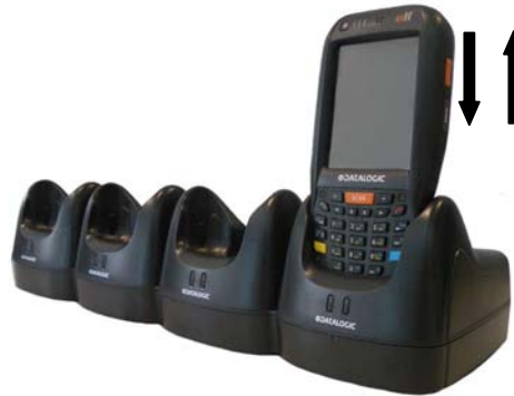
Figure 2 - Mobile Computer Insertion
