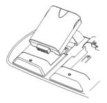
Caution! It is important that battery packs are inserted into the charging pocket correctly. Inserting the battery incorrectly could result in damage to the battery pack or the charger.
