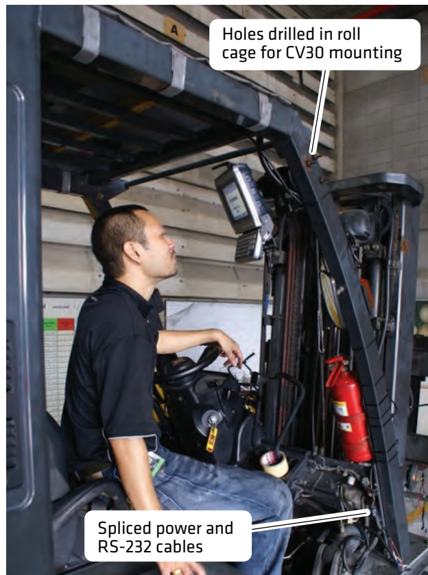
VMU Mounting: Holes were drilled in the roll cage for VMU mounting. Note splices in cable.
