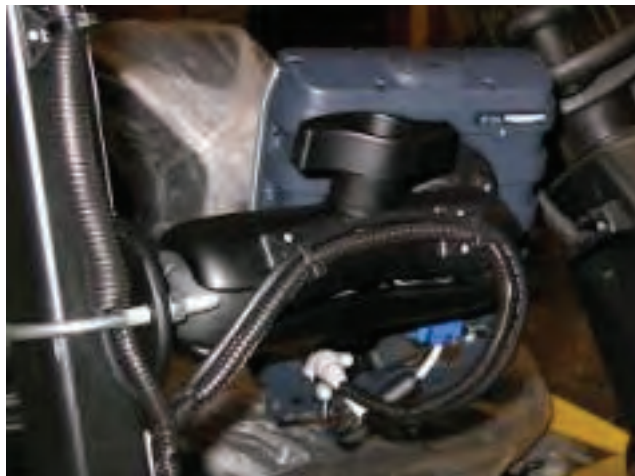
CV30 Horizontal Mounting: A single U-bolt holds the VMU mount to the roll cage. Poly sheath and Velcro fasteners provide a finished, professional look.
