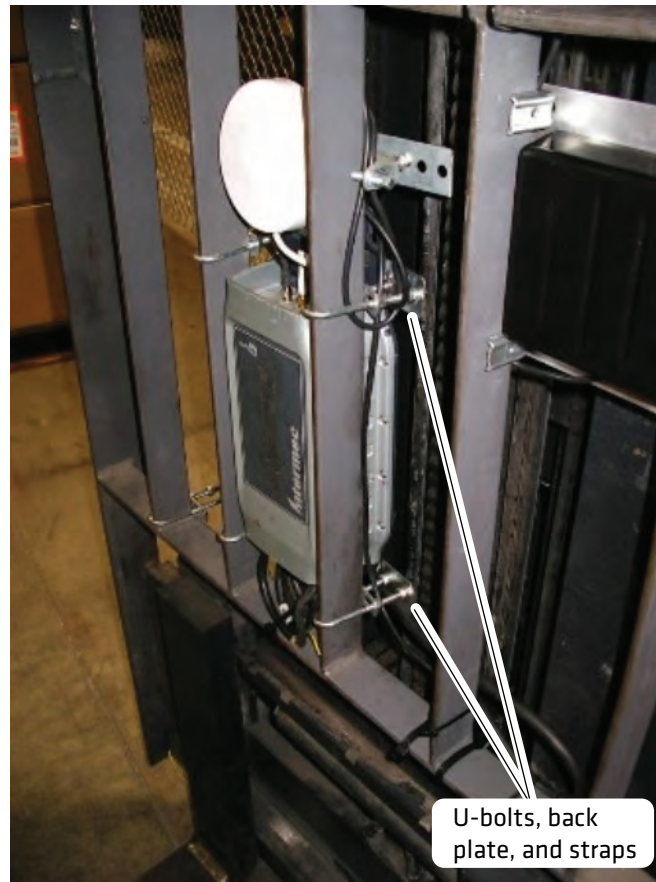
Prototype Antenna Mounting: Prototype installation before release of the Forklift Installation Kit (P/N 203-769-001)
