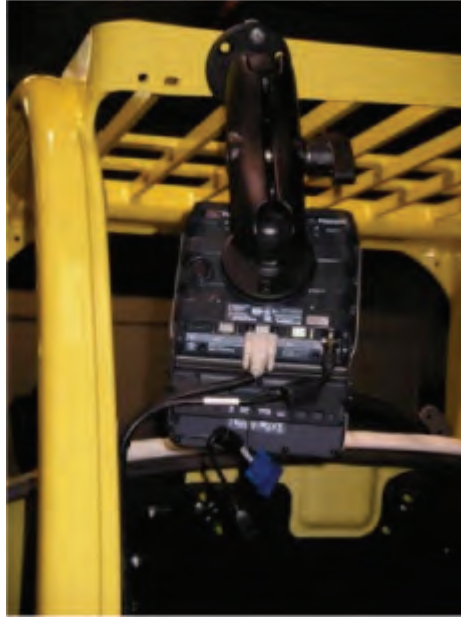
Mounting to Top of Roll Cage: VMU mount is secured with U-bolts.
