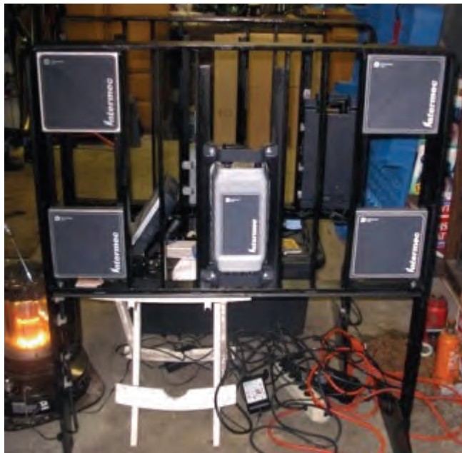
IV7 and Multiple Antennas: 4-antenna installation with IV7 in center channel of ALBR and antennas in end channels.
