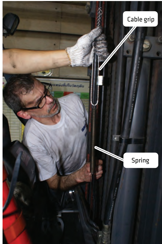
Cable Grip and Spring Installation: This cable grip and spring provided tension on the cable section coming out of the mast to the lift truck chassis.
