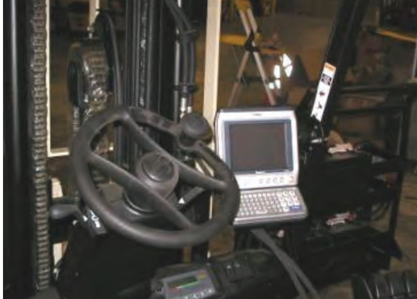
CV30 Horizontal Mounting: Driver's field of vision is clear with the CV30 mounted at this height.
